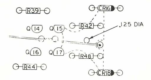
c. Fabricate circuit shown in Figure 1, above, on 3/4" x 1" perf board, using Figure 3, below, as a guide.
