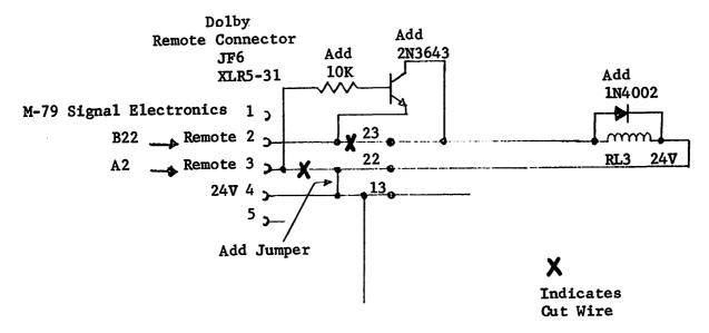
NOTE: Added Circuit may be mounted on a Vector Board inside the DOLBY unit.
