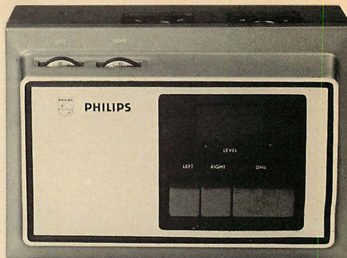
Fig. 3 —The DNL circuit, four transistors, six diodes, and a handful of common components, can easily be made up into a neat set-side box—no bigger than a double pack of 20 cancer-sticks.
