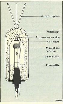
Fig.1. 1/2" Microphone and Preamplifier fitted with Rain Cover UA 0393 and Dehumidifier UA 0308, mounted inside the Windscreen UA 0570
