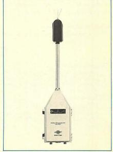
Fig.2. The Outdoor Microphone Unit Type 4921
