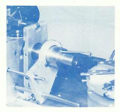
RETRACTING OUTER BARRIER—The device illustrated above consists of a tube concentric with the main spindle which is used to support the outer flange of the bobbin or the outer end of the mandrel. A bracket is mounted behind the "flyer" assembly and this is actuated so as to retract the barrier prior to the indexing of the turret.
