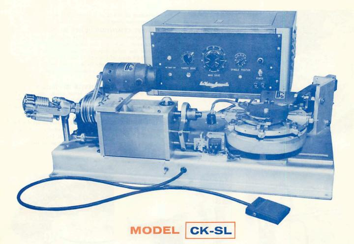
This machine differs from the Model CK at left only in the type of control circuit and in the fact that it has a reset mechanism which permits the cam to revolve 360° for each coil. It is specifically designed for close-wound or space-wound single-layer coils with either linear or non-linear turns' spacing. The wire spacing is determined by change gears and the number of turns is precisely controlled by measuring the coil length.
