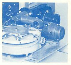
HOT AIR DRYING UNITS—Forced hot air is directed at the coils at two stations around the turret to accelerate drying of the cemented area. Dual heater and blower units with duct openings at four stations can be provided when faster drying is required.
