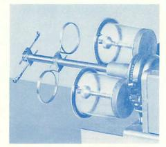
BIFILAR ATTACHMENT—This device rotates the spools of wire with the winding spindle so as to eliminate twisting of the strands of wire. Some reduction in machine speed is necessitated by the inertia of the wire spools, and it is therefore important to realize that many coils wound with two strands of wire simultaneously do not require this device.
