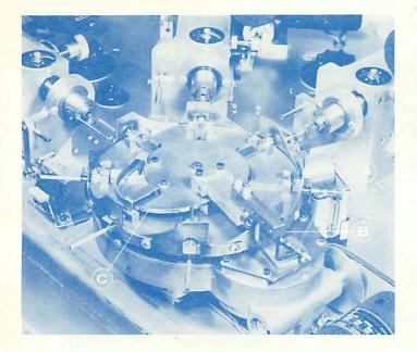
The illustration at left is of a three-head turret-type winding machine incorporating the following three attachments:
