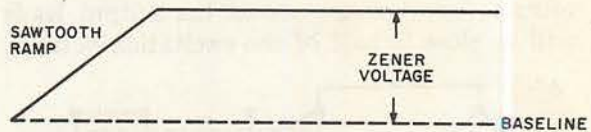
Fig. 2. Resultant Zener display allows several functional characteristics to be determined.
