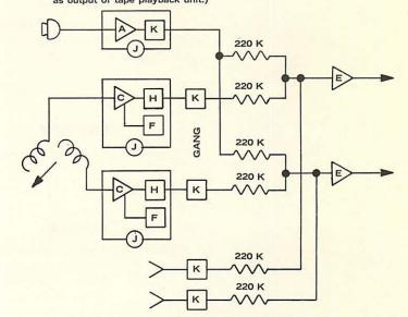
(NOTE: Undesired cross-channel signals will be more than 30 DB below program, under worst conditions. There will be no cross-channel with mic. gain closed).
