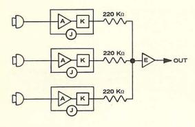
(4) MONOPHONIC (Split) MICROPHONE AND STEREO PHONOGRAPH (With aux. input for stereo source such as output of tape playback unit.)
