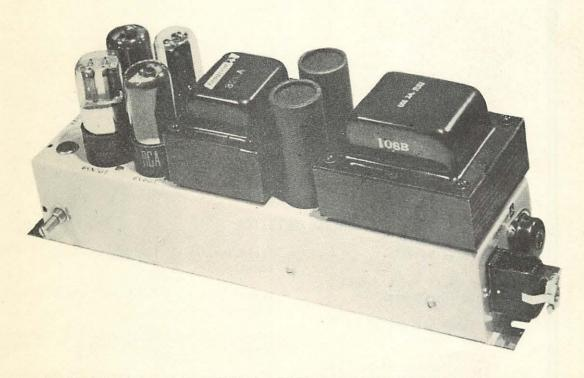
The small size of the I30A Amplifier permits mounting in consoles and cabinets or directly in the monitor speaker housing. Where several of the I30A Amplifiers are required, as in a rack installation, as many as four may be mounted on a standard Langevin IOB Mounting Frame.
