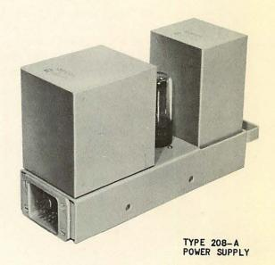
The chassis of the 208-A is constructed of 16 gauge steel which has been bonderized to prevent rust, and is finished in light grey baked-on enamel.
