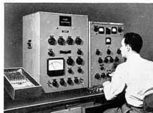
This precision inductor test is for a .3% reactor requiring precise high Q and accurate orientation in case.
