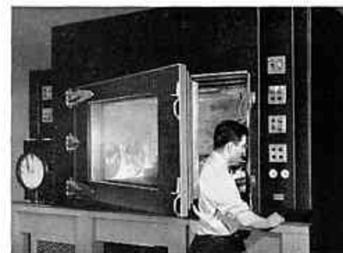
To assure dependability of hermetically sealed units, samples of production are run through controlled temperature and humidity cycling.
