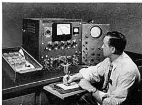
Magnetic Amplifier Testing. Five check points with DC controlled to .5%, inductance measured to .5%.
