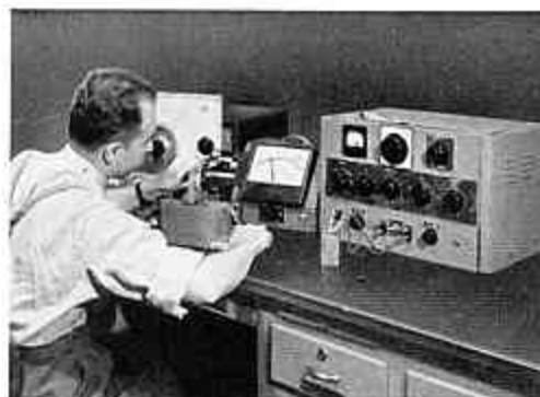
Phase angle and inductance checked to .05 degrees. Deviation cannot exceed .02 degrees from -40^{\circ}\text{C.} to +85^{\circ}\text{C.}
