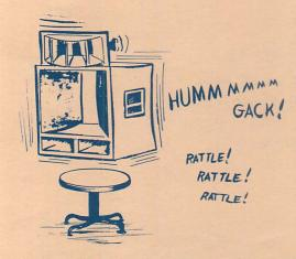
6. Avoid ground loops; ground loops and high power amplifiers may be fatal to loudspeakers. Do not make connections to equipment with levels up or power amps on. Use connectors that make ground connections first such as XLR type. Keep cables in good repair.
