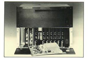
Altec Lansing's patented Model 2200 Incremental Power System is a power amplifier that lets you select components to create your own custom-made power system. Housed in a 7-inch high card-cage mainframe, the Model 2200 accommodates up to eight 75 watt (or four 150 watt) power amplifier cards, one or two electronic crossover cards, a balanced or unbalanced input card and special driver amplifier cards with matrix switching for console-like signal processing.
