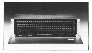
complete equalization bypass when the AC power switch is off, or when power to the unit is lost. The peak indicator on the front panel illuminates when the output level reaches +16 dB. Turn on/off transients are suppressed through output muting.
