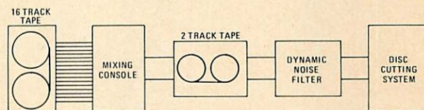
Fig. 2—Two-channel Dynamic Noise Filter reduces noise in a 16 track system.
