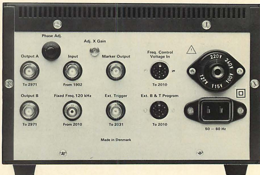
Fig. 8. Rear panel of TDS Control Unit showing sockets, the "Phase Adj." control and the "Adj. X Gain" potentiometer
