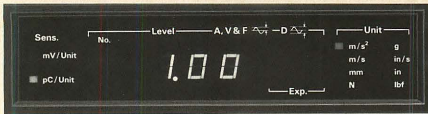
Fig. 1. Vibration meter LED display showing the selected accelerometer charge sensitivity
