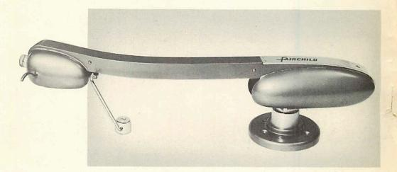
Fairchild, pioneer developer of the famed Turret-Head 3-Way Transcription Arm, now offers a highly improved version incorporating viscous damping in the lateral plane only. This means elimination of sluggishness, proper tracking of warped records and increased overall performance. A bi-metal unit is used to automatically insure proper lateral damping regardless of wide temperature variations.
