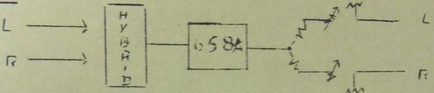
Mix left and right signal through hybrid (UTC LS 141) into the 658A. Check to be sure of adequate driving level. The hybrid must be tuned when installed.
