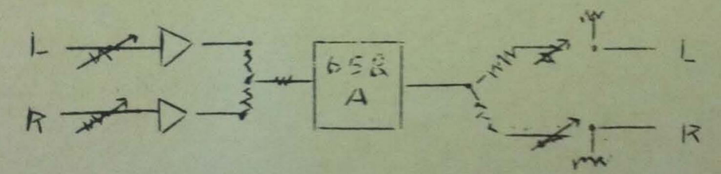
Feed left and right signal through level controls and amplifiers. The output should be mixed to feed through the 658A (200 ohm resistors - nominal 6 db loss). The output of the 658A is bridged as in Method A.
