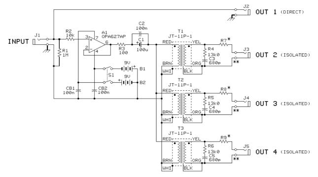
A LOWER COST OP—AMP, SUCH AS THE LF356N, MAY BE SUBSTITUTED FOR A1. ITS SLIGHTLY HIGHER NOISE (HISS) WILL BE INSIGNIFICANT UNLESS THE DC RESISTANCE OF THE PICKUP IS UNDER 3  $k\Omega,$
