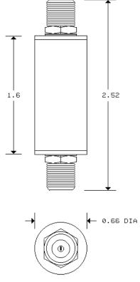
CONNECTORS ARE NICKEL PLATED BRASS "F" TYPE WITH GOLD PLATED CONTACTS
