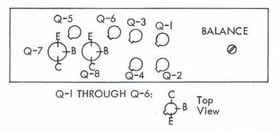
Adjust BALANCE control for minimum distortion at 30 cps. If distortion-measuring equipment is not available, adjust for zero voltage between the emitters of Q-5 and Q-6.
