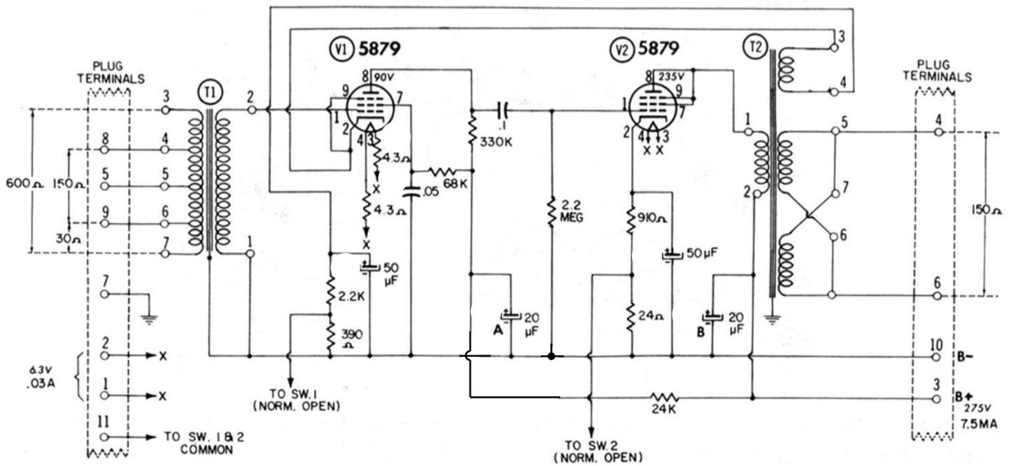
**Circuit diagram of Langevin type 5116 plug-in amplifier**
