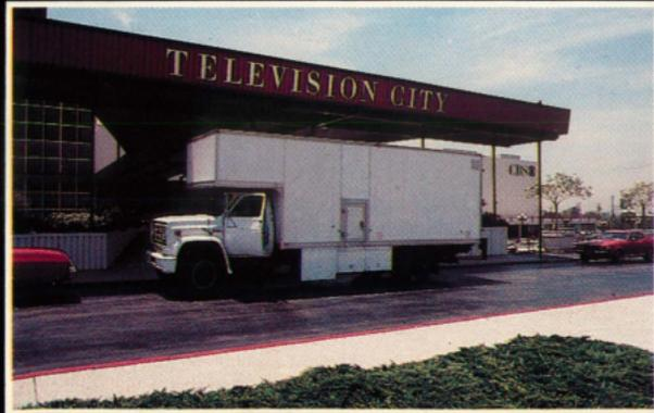
**TRUCK NUMBER ONE** 44X24 Automated Processes Console with: Simultaneous Quad-Stereo-Mono Mixdown. Grouping. Auto-mix. 88 Mic inputs. 2 M-79 3M 24-Track Recorders. 20X8 Air Conditioned Control Room. Closed Circuit TV w/ Color Monitor. 2-Channel Intercom. Wide Selection of Outboard Equipment. Mixers and Mics, SMPTE and Sync, Dolby.
