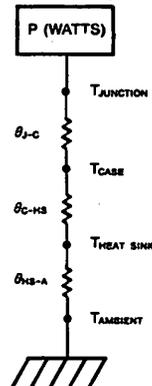
2. The thermal resistance from the power amp case to the heat sink,  $\theta_{C-HS}$ , depends on heat sink mounting surface flatness. Heat sink compound reduces  $\theta_{C-HS}$  in the presence of small surface imperfections. While it is not a substitute for good heat sink workmanship, it does conduct heat better than the air that would otherwise fill the voids resulting from surface irregularities.
