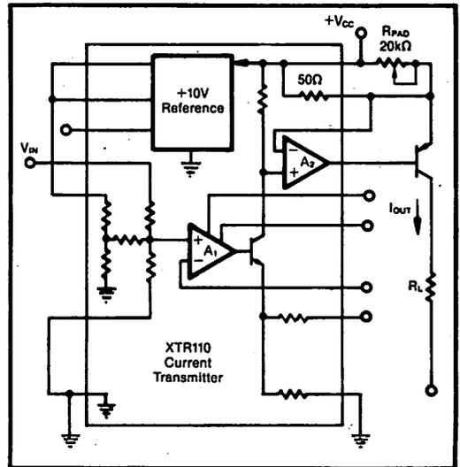
FIGURE 4. A fixed resistor or 20kΩ trimming potentiometer,  $R_{PAD}$ , corrects for variations in beta when a less costly PNP transistor is used instead of a MOSFET at the output of the current transmitter.
