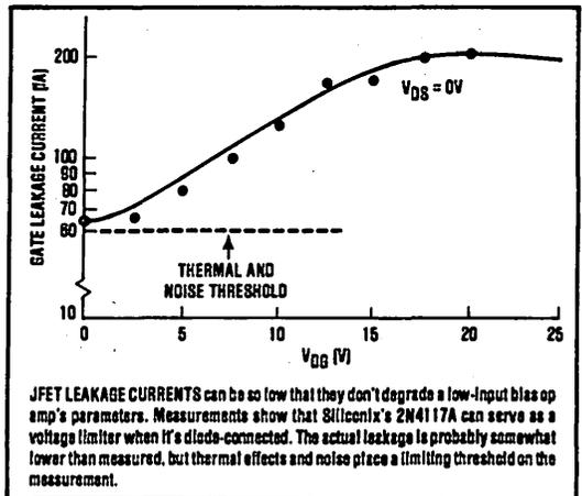
FIGURE 2. Curve of Leakage Current vs Voltage.
