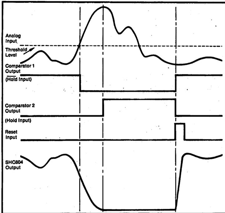
FIGURE 2. Timing Diagram.
