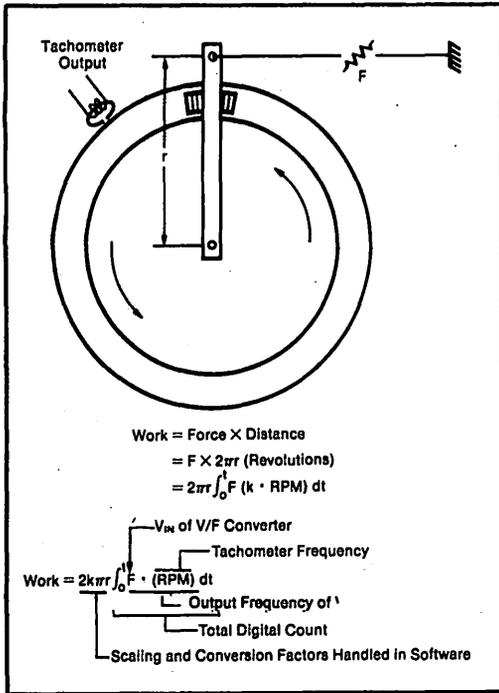
FIGURE 2. Instruments on the stationary bicycle measure the work done. The force required to restrain the brake assembly (which would otherwise be free to rotate with the wheel) is multiplied by the radius of the force, yielding the applied torque. The time integral of torque times speed is mechanical work.
