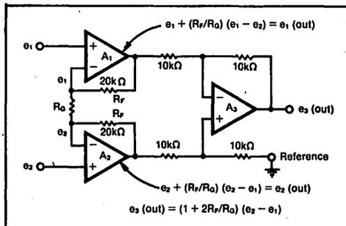
FIGURE 1. Two noninverting op amps with combined feedback, and a difference amplifier form an instrumentation amplifier with many design options.
