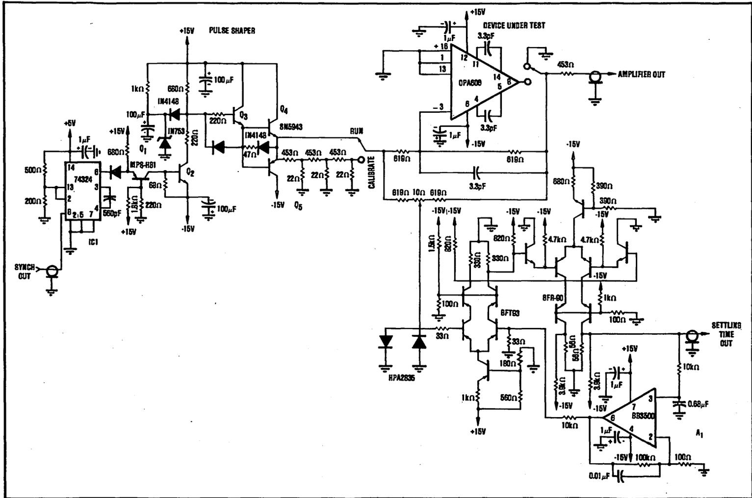
FIGURE 11. Settling Time Test Fixture for High Speed Operational Amplifier.
