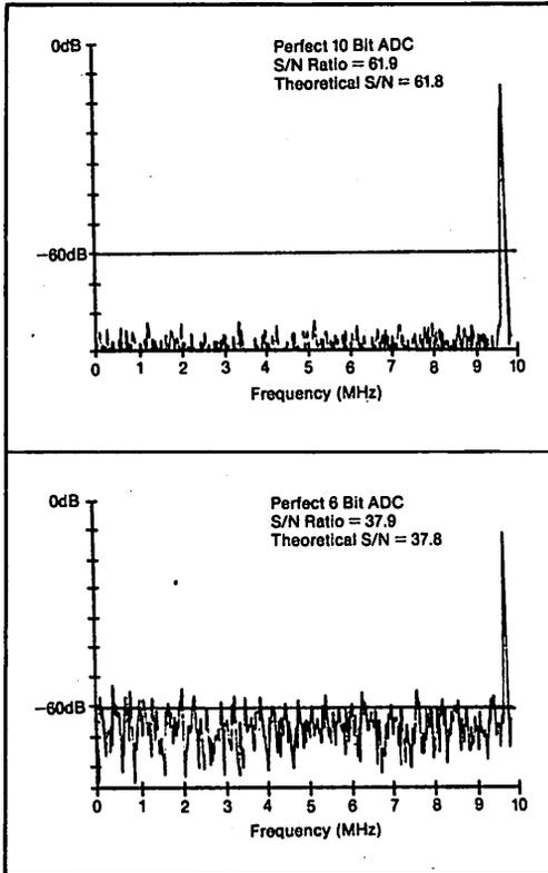
FIGURE 14. FFT plots for 0.85MHz data quantized by perfect 10-bit (top) and 6-bit (bottom) ADCs. The signal-to-noise ratio computed in each case agrees closely with the theoretical value of  $6N + 1.8\text{dB}$  where  $N$  is the number of ADC bits.
