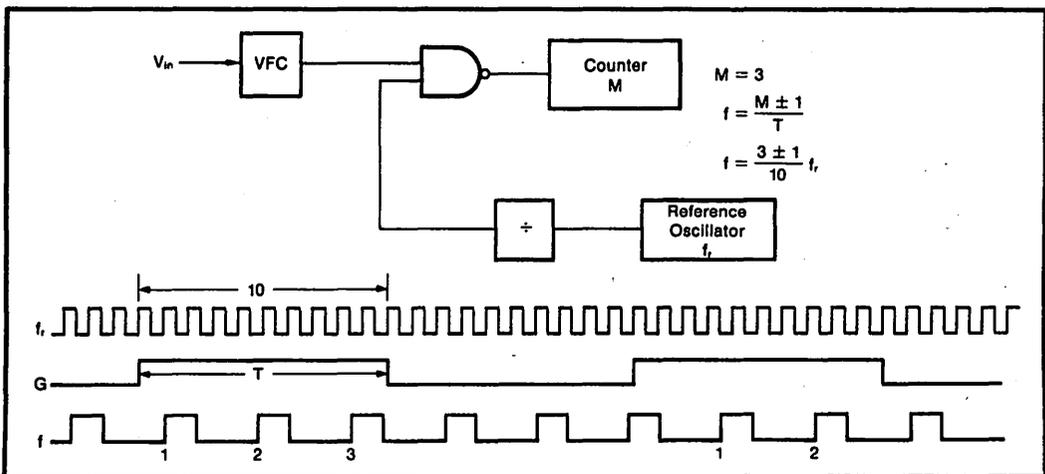
FIGURE 1. This simplified diagram of the standard counting method shows the potential inaccuracies that can occur. Although the first gate counts three rising edges of the VFC output frequency,  $f$ , the second gate period counts only two.
