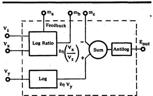
FIGURE 1. Multifunction Circuit Block Diagram.
