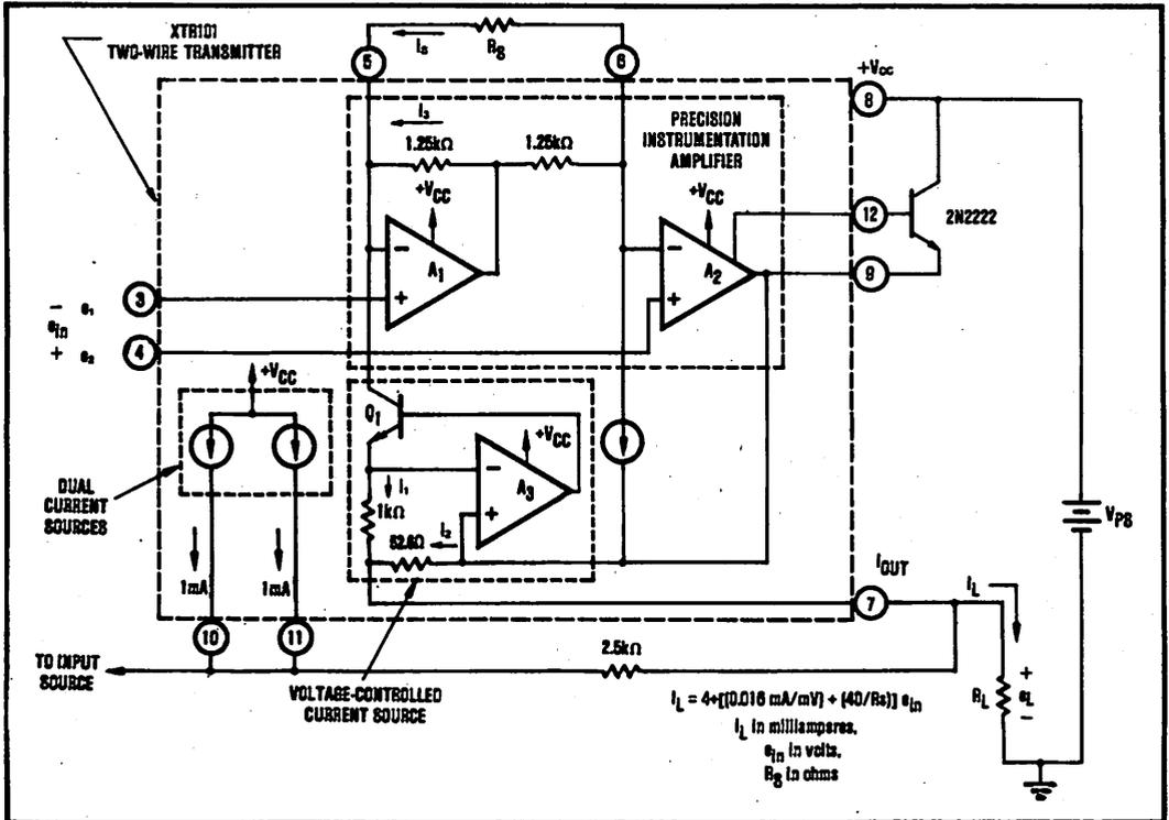
FIGURE 1. A two-wire transmitter in hybrid IC form, the XTR101 modulates the power supply current with changes in the input voltage,  $e_{in}$  (at pins 3 and 4). In addition, the circuit contains two 1mA current sources for powering transducers.
