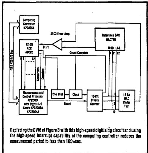
Replacing the DVM of Figure 3 with this high-speed digitizing circuit and using the high-speed interrupt capability of the computing controller reduces the measurement period to less than 100µsec.
