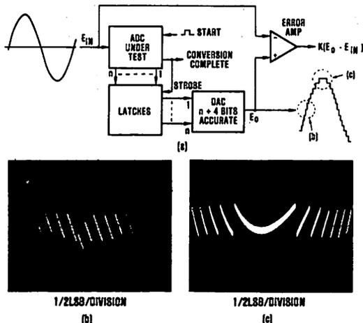
FIGURE 8. ADC Test Circuit. (a) Comparing  $E_{in}$  and the ADC output which is converted back to an analog voltage with an accurate DAC. (b) Error at  $E_{in} = 0$ . (c) Error at plus full-scale input.
