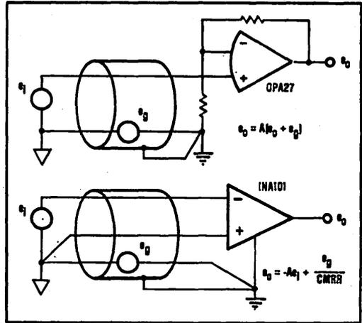
FIGURE 1. While an Op Amp (top) Amplifies a Ground-Line Signal ( $e_n$ ), an Instrumentation Amplifier (bottom) Attenuates It.
