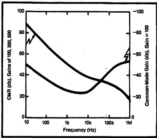
FIGURE 3. You can improve the common-mode rejection for worst-case mismatches of time constants  $R_1C_1$  and  $R_2C_2$  in the Figure 2 circuit by adding a small trimming resistor in series with  $R_1$  and  $R_2$ .
