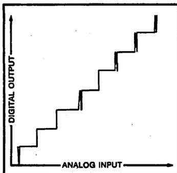
FIGURE 5. A portion of the transfer function for an ADC71KG converter with 14-bit resolution—operating at the specified maximum conversion time of  $50\mu\text{s}$ —shows inherent noise at transition points.
