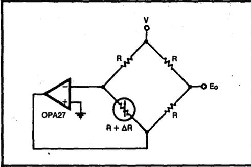
Unfortunately, this circuit provides no amplification and doesn't accommodate heavy loading. Output resistance equals  $R/2$ , and heavy loading significantly attenuates the output signal. But these limitations present no problems if you're interfacing with a data-acquisition system that has its own input amplifier or where bridge output signal is sufficiently large to directly drive an A/D converter.
