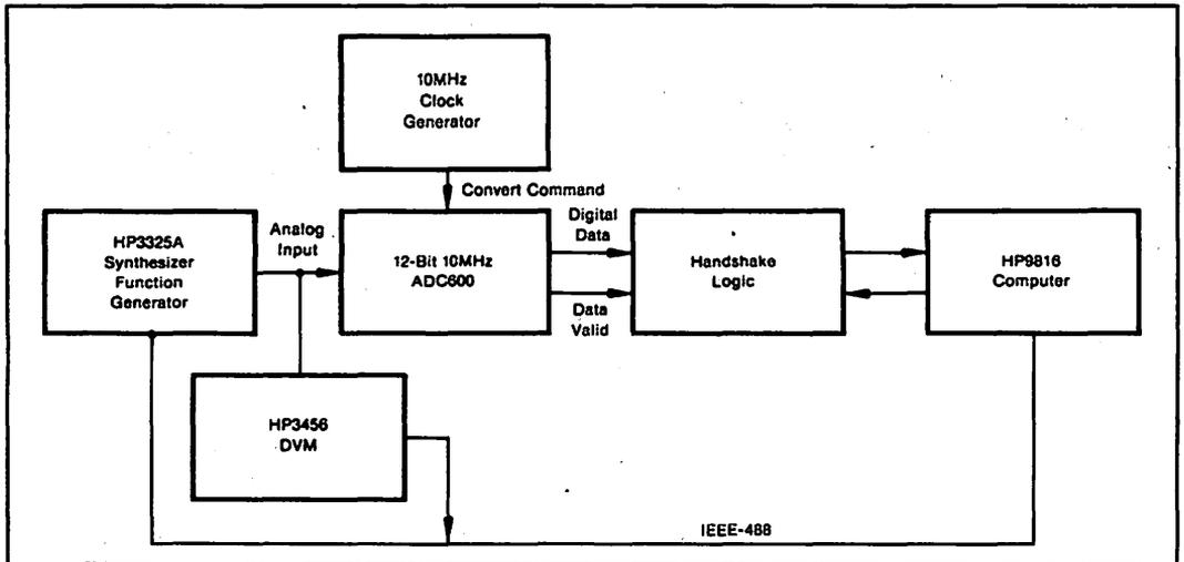
FIGURE 11. Block Diagram of Histogram Test.
