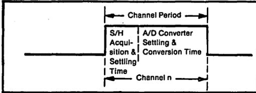
FIGURE 6b. System Throughput Rate - Overlap Mode.
