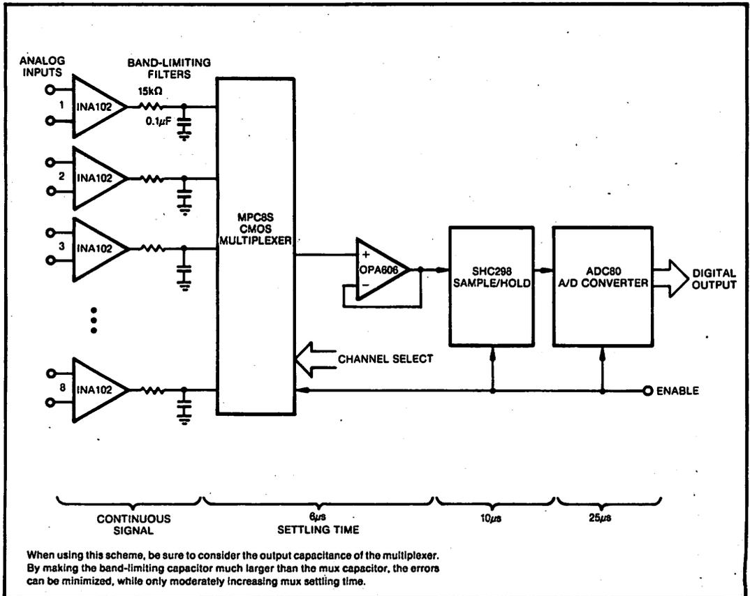
**FIGURE 5.** You can increase the throughput rate of a data-acquisition system by dedicating an INA102 to each analog input channel. In this example, rates can approach 24,000 samples-per-second.
