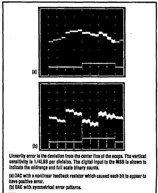
Linearity error is the deviation from the center line of the scope. The vertical sensitivity is  $1/4\text{LSB}$  per division. The digital input to the MSB is shown to indicate the midrange and full scale binary counts.
