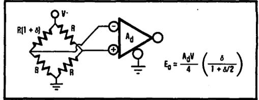
FIGURE 8. Bridge Amplifier with One Active Bridge Arm.
