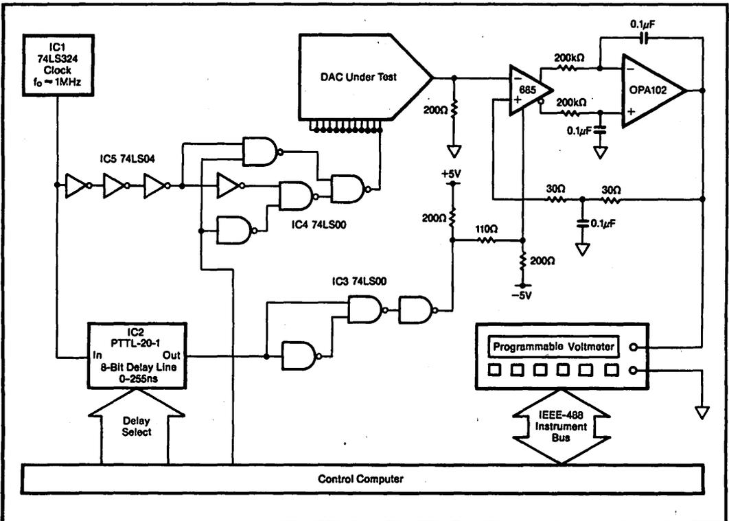
FIGURE 6. Simplified Schematic of the DAC Tester.
