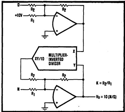
FIGURE 3. More Accurate. The multiplier-inverted divider exhibits improved accuracy when connected in the manner shown. The error equation is given approximately by  $e_d = 10e_m(KD)$ , where  $K$  is the ratio of  $R_2$  to  $R_1$  and can be used to optimize the divider's range.
