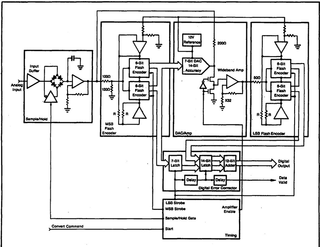
FIGURE 2. Block Diagram of 12-Bit 10MHz ADC600.
