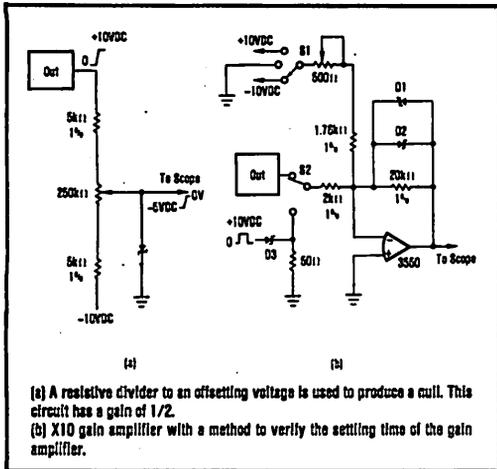
FIGURE 6. Circuits for Measuring Settling Time.
