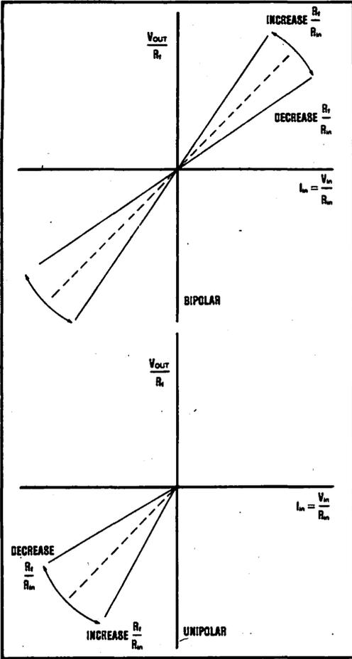
FIGURE 8. ADJUSTING THE GAIN. Changing the ratio  $R_f/R_{in}$  will change the gain by rotating the transfer function about the point where  $I_{in} = 0$ . This will be true for both the unipolar and bipolar cases.  $I_{OS}$  is zero in these examples.
