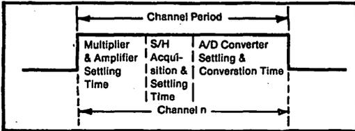
FIGURE 6a. System Throughput Rate - Serial Programming.
