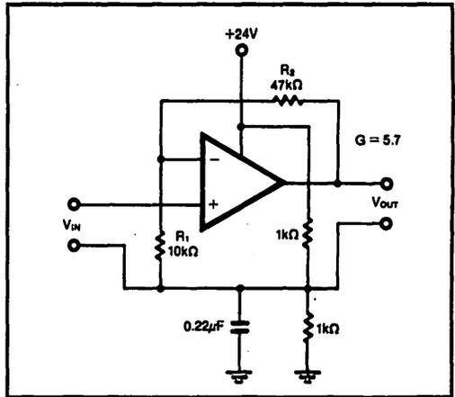
FIGURE 5. Even though the impedance of the voltage divider is in series with  $R_1$  to ground, the gain of this noninverting circuit is determined solely by  $R_1$  and  $R_f$ . Since the input and output are referenced to the same floating ground, its impedance does not affect the voltage gain of the circuit.
