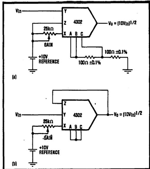
FIGURE 7. Another Approach. the multifunction converter (here, the 4302) may also be used as a square-rooter. To implement the transfer function,  $V_o = X(YZ)^m$ ,  $m$  can be equal to 1/2 (a) or to 1 (b), with the other connections appropriately made.
