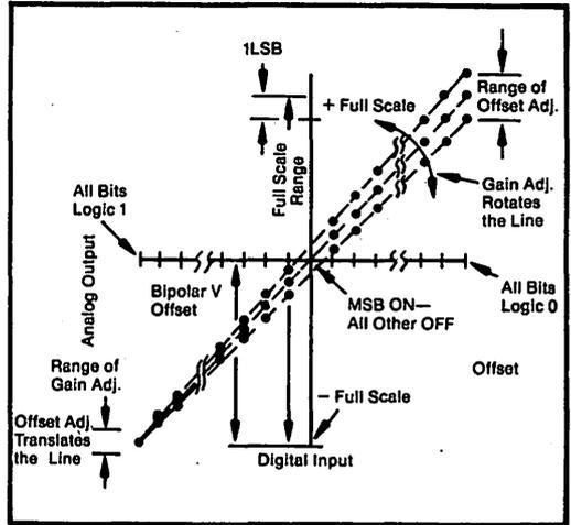
FIGURE 2a. DAC Gain Adjust Rotation Using GAIN ADJ Pin.
