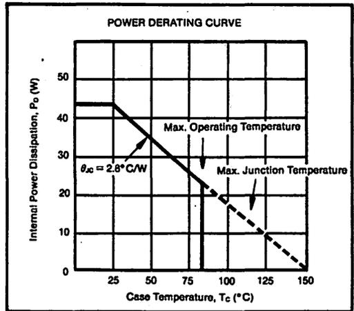
FIGURE 9. The power derating curve indicates that internal dissipation must be reduced at case temperatures greater than  $+25^{\circ}\text{C}$ . This reduces the available SOA in the power and second breakdown regions.
