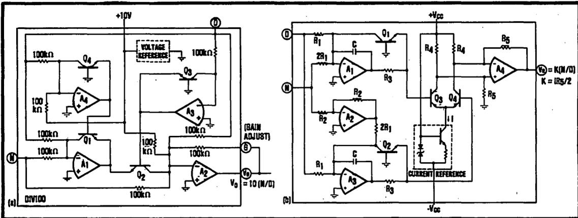
FIGURE 5. Divider IC. The four op amps and the four logging transistors shown in the functional diagram (a) are rearranged and the voltage reference is replaced by a current reference to form a log-antilog divider that maintains a constant-level bandwidth with decreasing divisor voltages (b).
