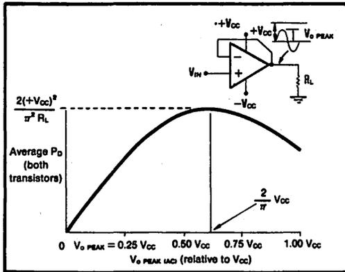
FIGURE 8. The average dissipation under continuous AC signals is a function of the output voltage relative to the supply voltage. Peak dissipation occurs at a peak AC voltage of approximately  $0.6V_{CC}$ . Unlike the DC case, the dissipation does not approach zero at maximum output voltage, but drops to roughly one-half its highest value.
