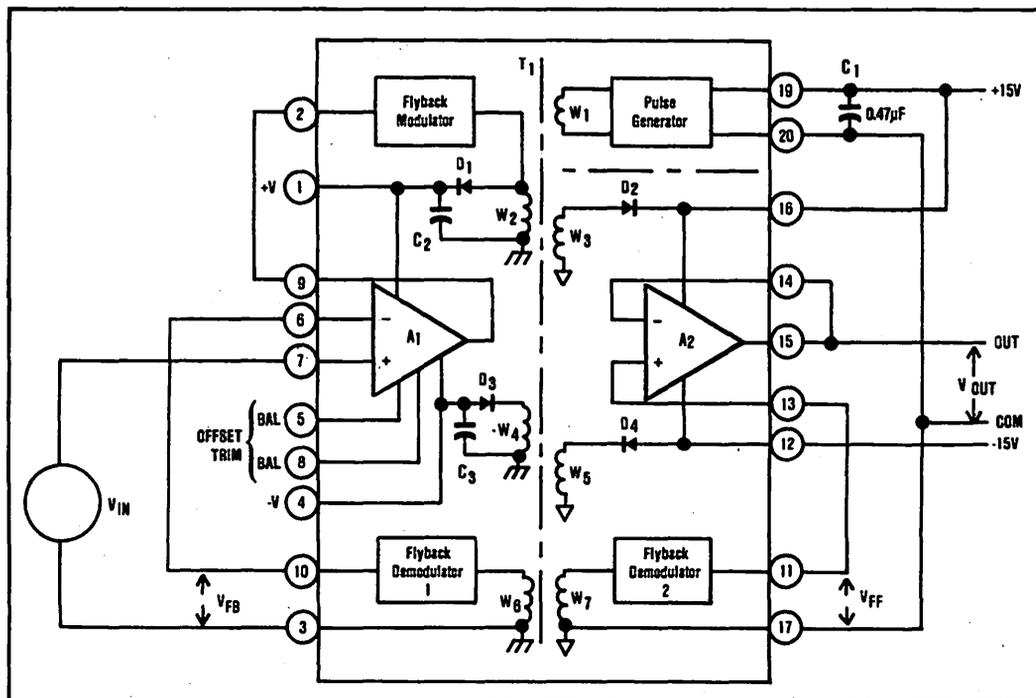
FIGURE 1. Self-contained by design. Functional diagram of hybrid isolation amplifier shows transformer  $T_1$  at its heart and a minimum of external components. Switching rate of 750kHz results in high frequency response and eliminates external filter components.
