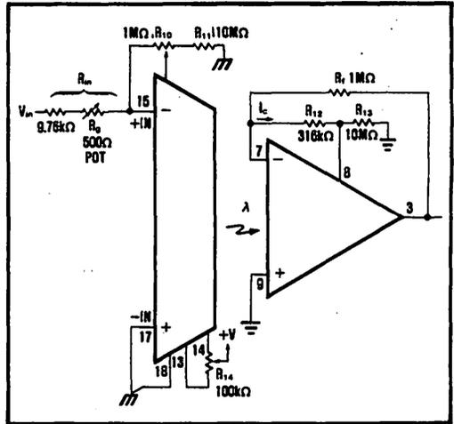
FIGURE 12. ADJUSTING THE BIPOLAR ERRORS (EXAMPLE 4). Each of the errors are adjusted in turn. With  $V_{in} = \text{"open"}$ ,  $I_{Os}$  is trimmed by adjusting  $R_{I0}$  to make the output zero.  $R_9$  is then adjusted to trim the gain error. The effects of offset voltage are removed by adjusting  $R_{I4}$ .
