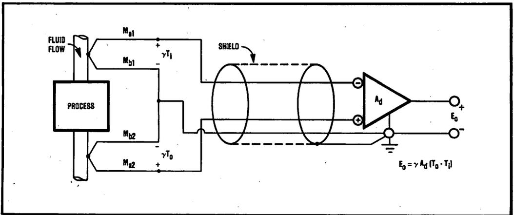
FIGURE 10. Differential Temperature Measurement with Two Thermocouples formed by Metals  $M_a$  and  $M_b$ .
