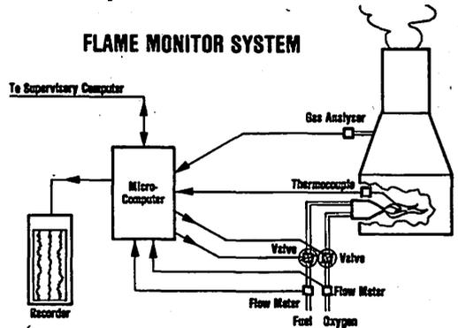
FIGURE 1. A microcomputer monitors and controls a combustion boiler. Inputs from flame temperature transducers, effluent gas analyzers and fuel flow meters are monitored by the microcomputer. Using the inputs to compute the control algorithm, it adjusts the valves controlling fuel and oxygen and also drives a small strip chart recorder.
