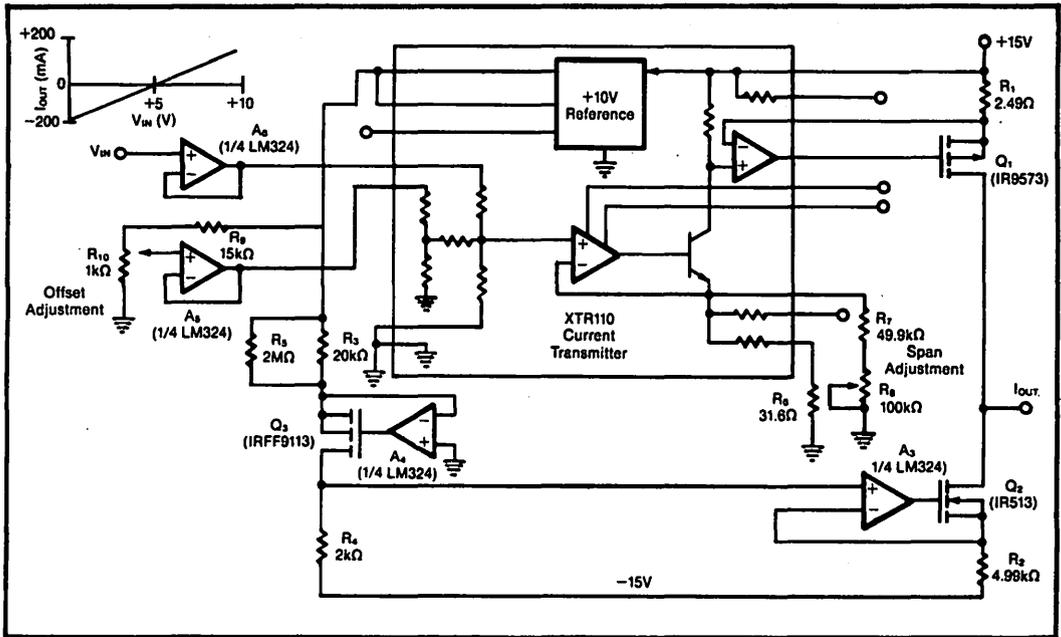
FIGURE 5. Alterations to the support circuitry to the current transmitter allow it to accommodate actuators that require a bipolar current. Resistors  $R_1$  and  $R_2$  feature low temperature coefficients and dissipate just 0.2W continuously;  $R_6$  and  $R_{10}$ , two 10-turn potentiometers, afford great sensitivity.
