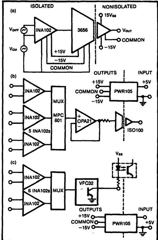
FIGURE 1. You can achieve high-performance isolated signal acquisition by exploiting the INA102's low current requirements. You can interface the INA102 directly to an isolation amp (a) or an 8-channel CMOS multiplexer (b). Another circuit (c) provides an easy technique for analog-to-digital conversion.
