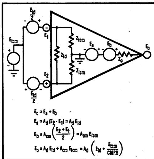
FIGURE 1. Model of Instrumentation Amplifier
