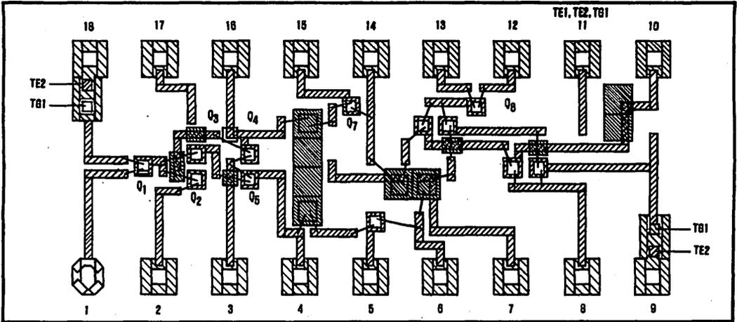
FIGURE 2. Layout of Hybrid Assembly for Wideband Amplifier.
