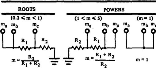
FIGURE 2. Exponent Selection for Multifunction Circuit. Resistors  $R_1$  and  $R_2$  from a voltage divider. For  $m$  less than one, the log ratio output is simply attenuated by  $R_1$  and  $R_2$ . For  $m$  greater than one,  $R_1$  and  $R_2$  determine the gain of the log ratio amp.
