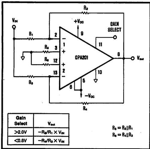
FIGURE 7. Selectable-Gain Amplifier.
