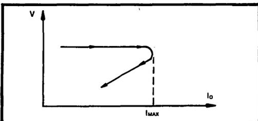
FIGURE 12. Foldback Circuit.
