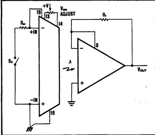
FIGURE 10. PREFERRED METHOD FOR VOLTAGE OFFSET TRIM. In those rare applications where offset voltage is significant, it is best to adjust the input offset voltage,  $V_{OSi}$ , as shown above.  $V_{OSi}$  and its drift appear at the output multiplied by the factor  $R_f/R_{in}$ .  $V_{OSi}$  will usually not be gained up, and thus will not need adjustment. Adjust  $V_{OSi}$  until opening up and closing  $S_1$  causes no shift in the output voltage.
