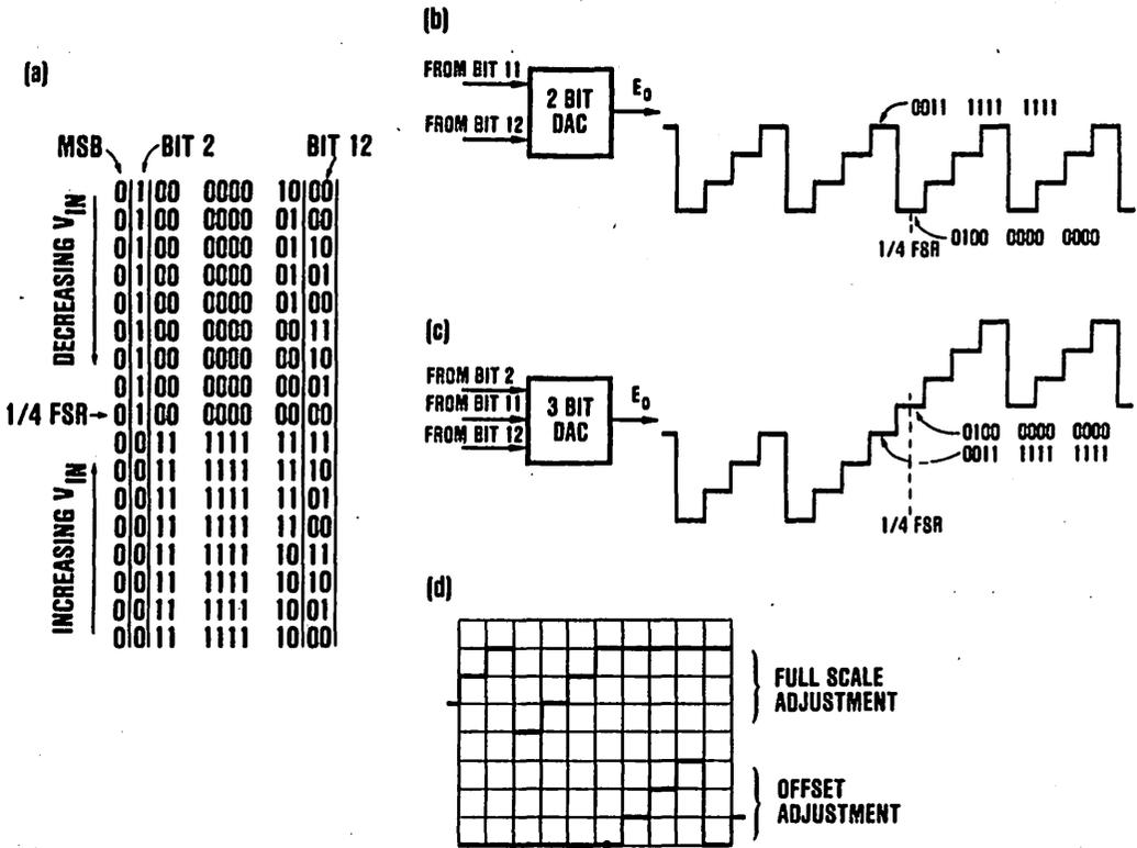
FIGURE 6. Basis for the Dynamic Transfer Function Tester of Figure 5. (a) Repeating binary codes in the last two bits of an ADC output code for an input dither voltage at 1/4 of the full-scale range voltage. (b) Staircase waveform from a 2-bit DAC. (c) Shifted staircase waveform when the MSB of a 3-bit DAC is connected to the appropriate output of the ADC. (d) Offset and full-scale adjustments prior to examining the ADC transfer function.
