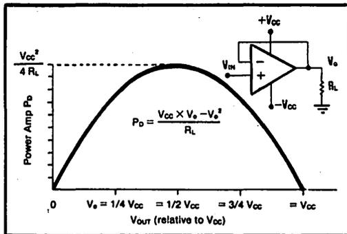
FIGURE 6. The power dissipation for a simple resistive load and DC input signal is at a maximum when the output voltage is  $V_P/2$ . Despite the larger currents at higher output voltages, the dissipation is actually lower. It approaches zero as the  $V_{CB}$  nears zero at maximum output voltage.
