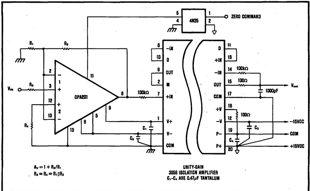
FIGURE 6. Software Auto-Zeroing the 3656 Isolation Amplifier.
