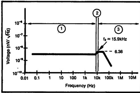
FIGURE 9. Output Voltage Due to Noise Current.
