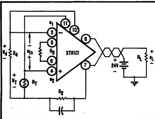
FIGURE 2. In applying the XTR101 in a temperature-measuring circuit, the operating point is fixed by the span resistance,  $R_s$ , a zero-suppression voltage across  $R_s$ , an input biasing voltage across  $R_s$ , and of course the resistance of the RTD.
