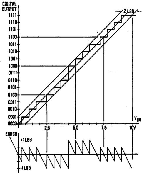
FIGURE 3. Transfer Function and Error Plot for an ADC which Contains a DAC with Individual Bit Errors of  $\epsilon_1 = -1/2LSB$ ,  $\epsilon_2 = +1/2LSB$ ,  $\epsilon_3 = 0$ , and  $\epsilon_4 = 0$ .
