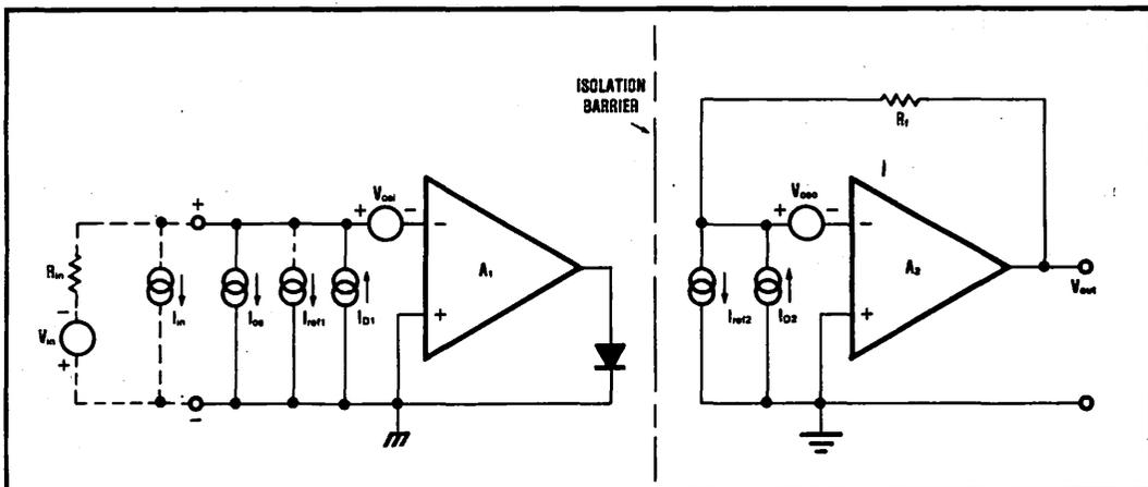
FIGURE 2. DC ERROR MODEL.  $V_{os1}$  and  $V_{os2}$  model the respective input offset voltages. There are several possible contributors to offset current. The composite effect is modeled with one current source,  $I_{os}$ , at the input. The gain error ( $A_e$ ) defines the relationship between  $I_{D1}$  and  $I_{D2}$  ( $I_{D2} = I_{D1}(1 + A_e)$ ). While shown as separate sources, any mismatch in  $I_{ref1}$  and  $I_{ref2}$  are included in the  $I_{os}$  term.
