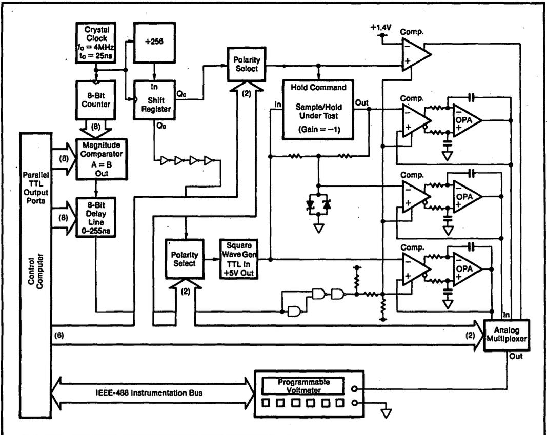
FIGURE 7. Simplified Diagram of the Sample/Hold Tester.
