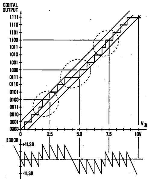
FIGURE 2. Transfer Function and Error Plot for an ADC which Contains a DAC with Individual Bit Error of  $\epsilon_1 = +1/2\text{LSB}$ ,  $\epsilon_2 = -1/2\text{LSB}$ ,  $\epsilon_3 = 0$ , and  $\epsilon_4 = 0$ .
