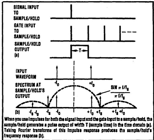
When you use impulses for both the signal input and the gate input to a sample/hold, the sample/hold generates a pulse output of width  $T$  (sample time) in the time domain (a). Taking Fourier transforms of this impulse response produces the sample/hold's frequency response (b).
