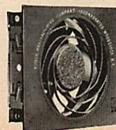
Fan assembly kit especially grouped for the home entertainment field, hi-fi/stereo, TV receivers, ham radio equipment, etc. Supplied with Whisper venturi fan electrical connector, mounting hardware and detailed instructions for mounting in three possible arrangements. Noise level only 18 db (SIL). For 105-120 VAC, 50-60 cps, single phase operation. Size, 4 1/4" sq. x 1 1/2" d. Weight, 1.2 lbs.
