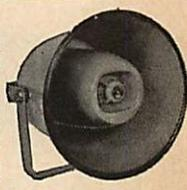
**Atlas Model W-6 Projector**—Similar to Model WT-6, but incorporates single driver. Used where extra-high frequency response is not required. **Power Input:** 15 watts, continuous duty. **Frequency Response:** 100-8,000 cps. **Impedance:** 8 ohms. **Dispersion:** 120°. **Shipping Weight,** 14 lbs. Net Each. . . . . \$27.00
